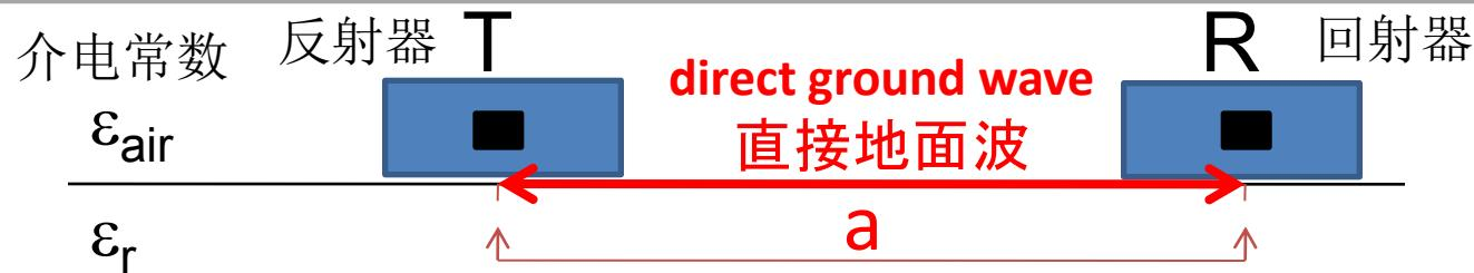
Near-surface soil moisture content from the ***direct ground wave signal***
